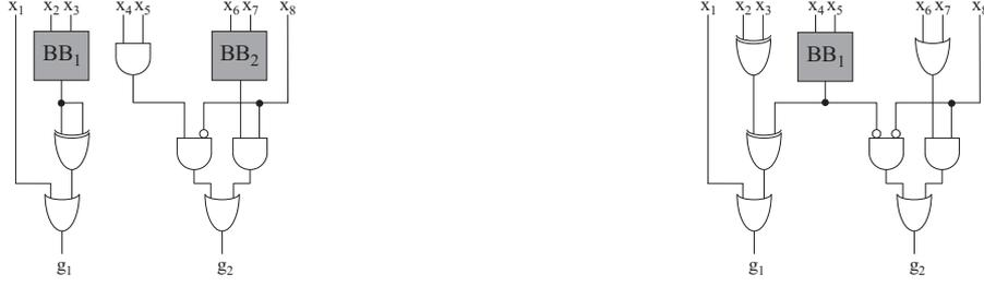
(a) Partial implementation with error detectable by  $Z_i$ -simulation, but not by  $Z$ -simulation
